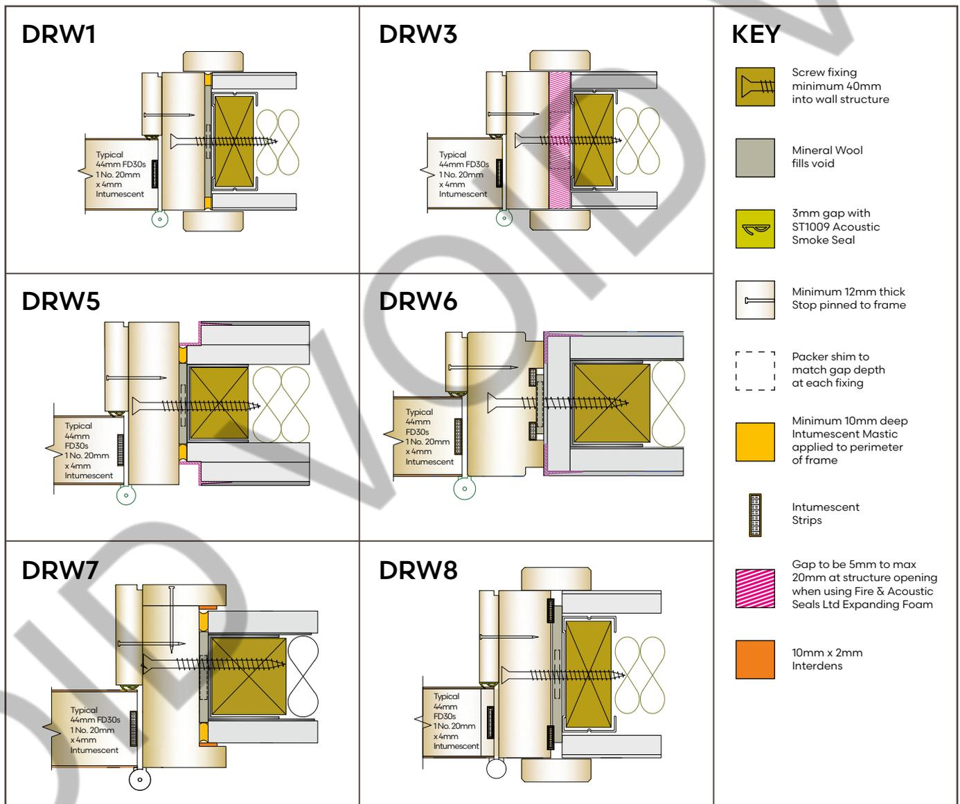
For all other gaps between the frame and the supporting construction (with or without architraves) the method of installation should follow the recommendations given in Section 9.4 of BS 8214:2016, "Timber based fire door assemblies - Code of Practice", using fire seal products proven in linear timber applications.
