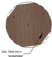
Hinge mortise repair, filled with Pyromas A intumescent mastic
