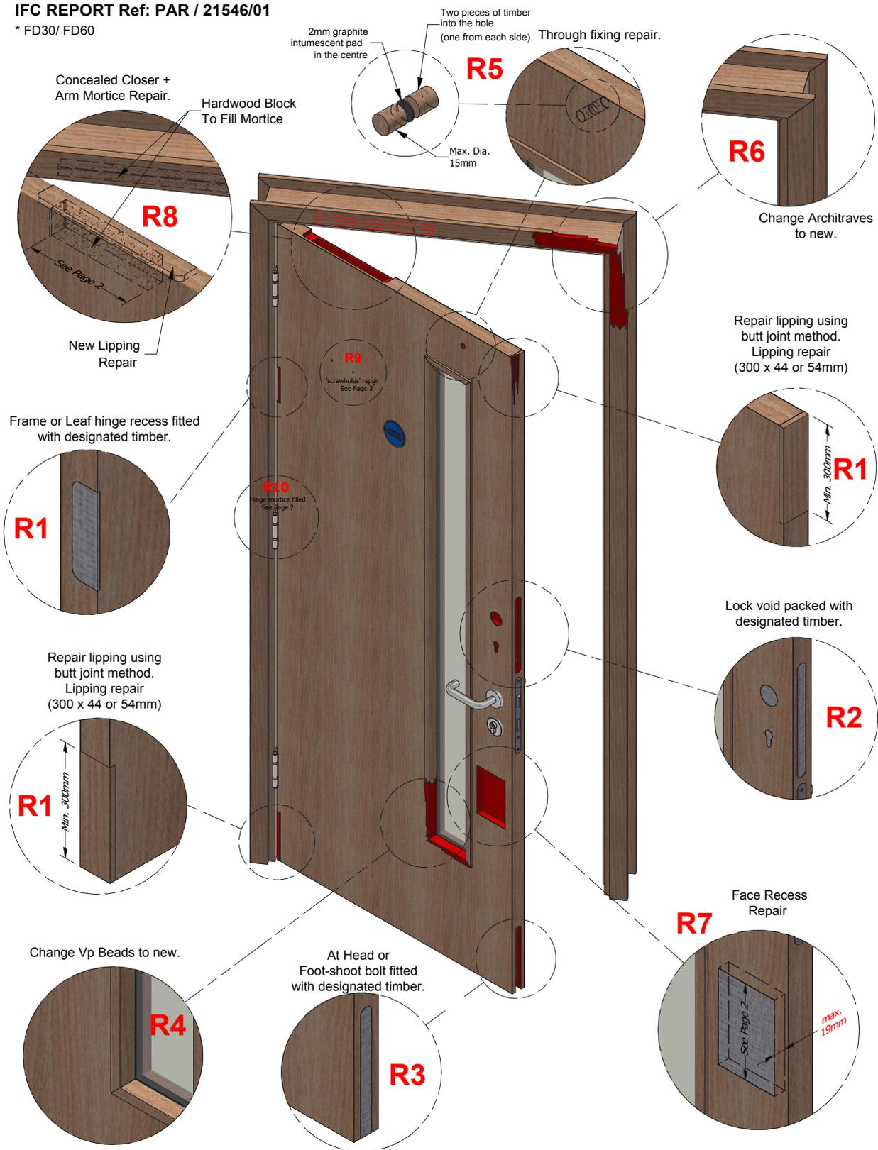
**FD30 min. Timber Density - 450 kg/m<sup>3</sup>**
