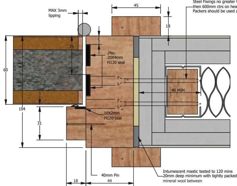
Steel Fixings no greater than 200mm from corners, then 600mm ctrs on head and stiles. Packers should be used at all fixing positions.
